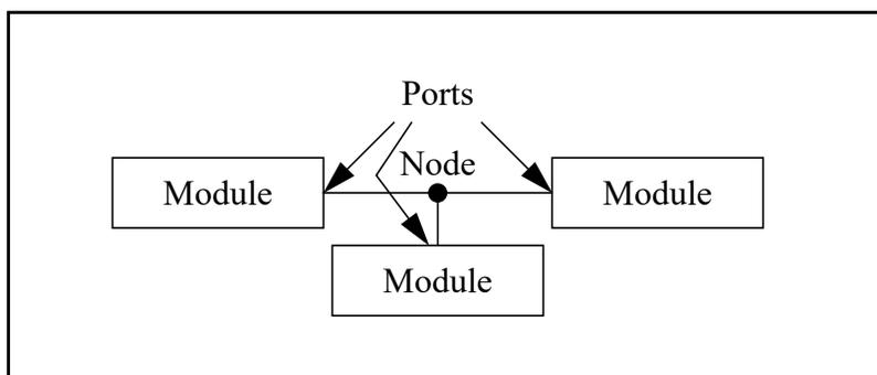
**Figure 1-1: Components connect to nodes through ports**
