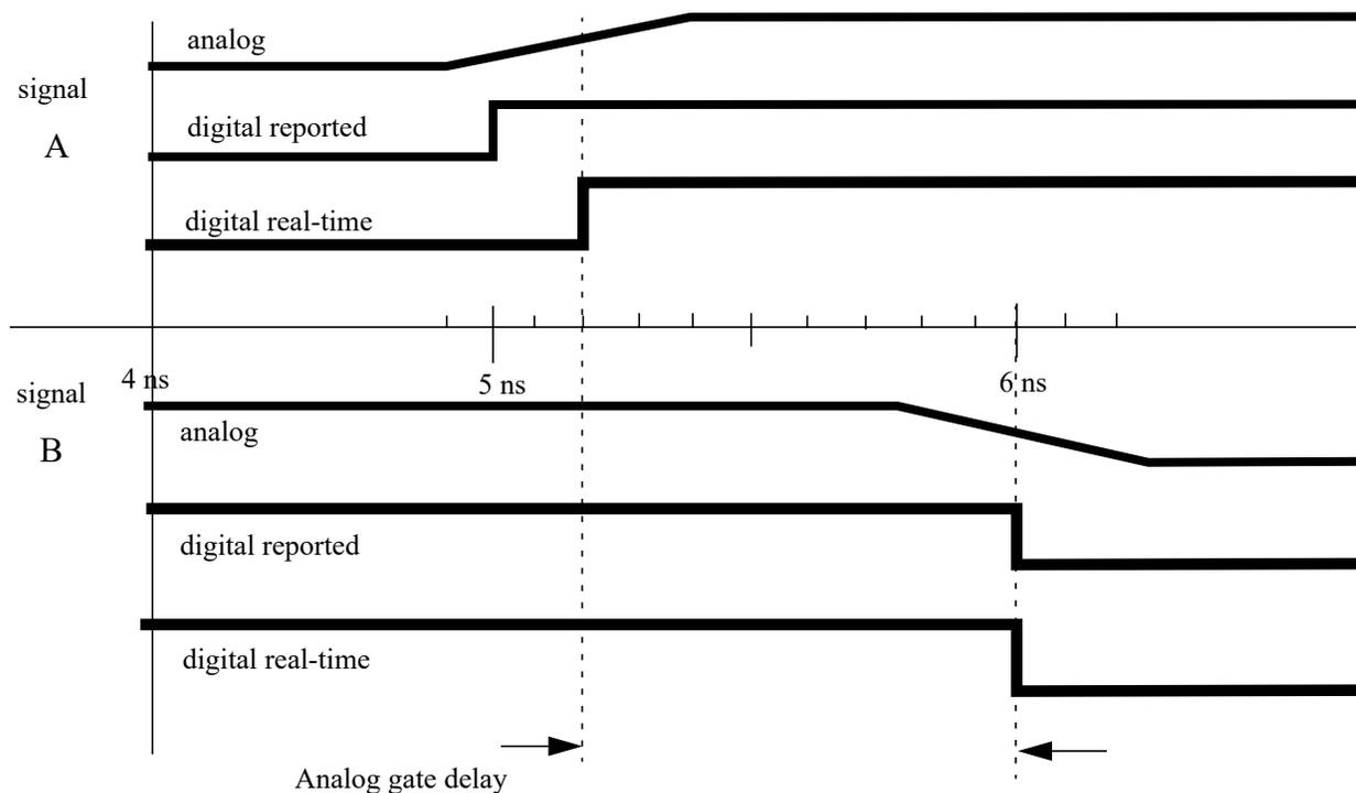
**Figure 8-5: Unit delay transient solution times**
