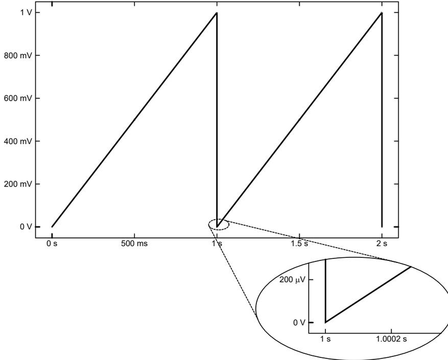
Figure 4-3: The output from the ramp generator
