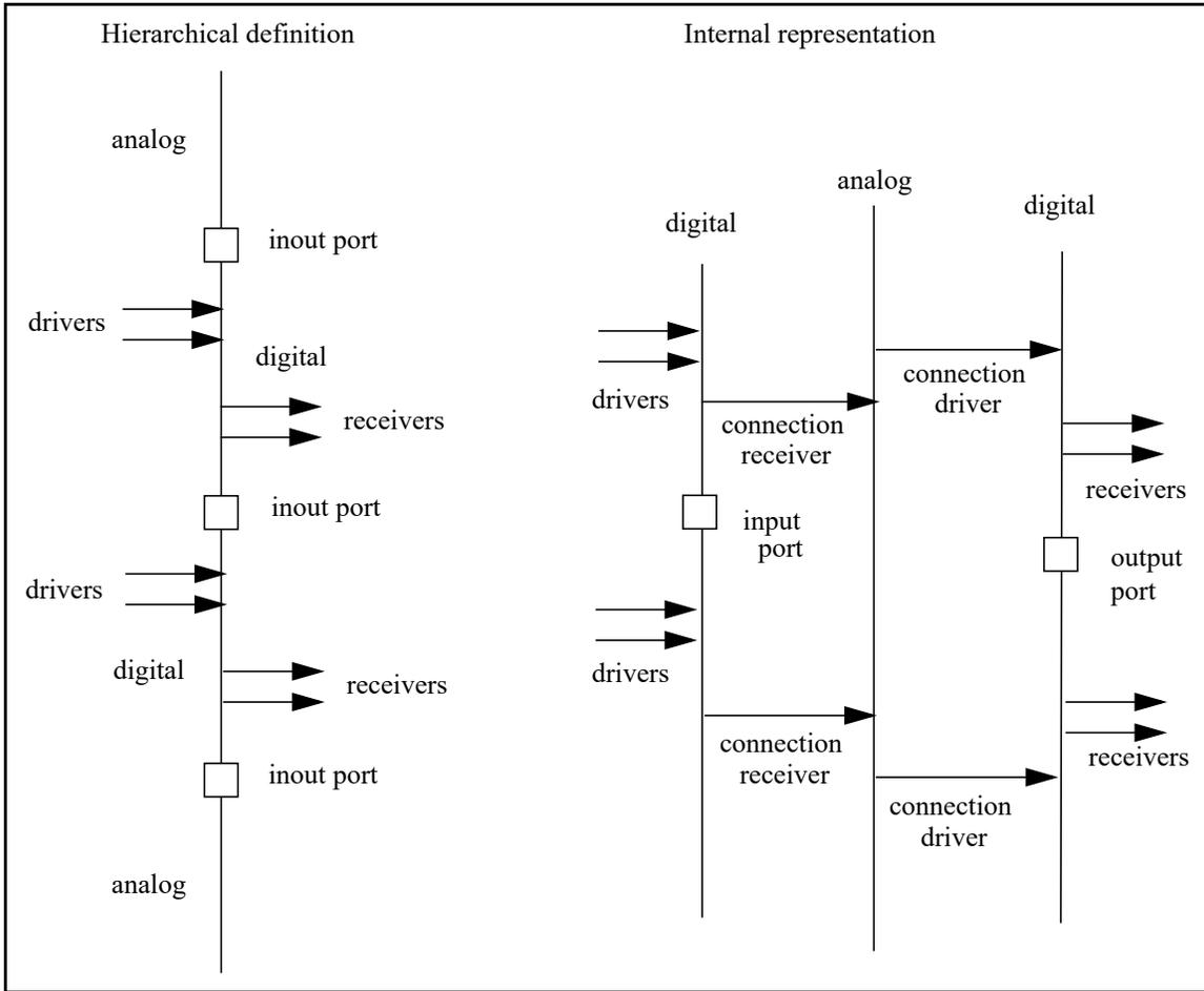
**Figure 7-11: Driver-receiver segregation in modules with bidirectional ports**
