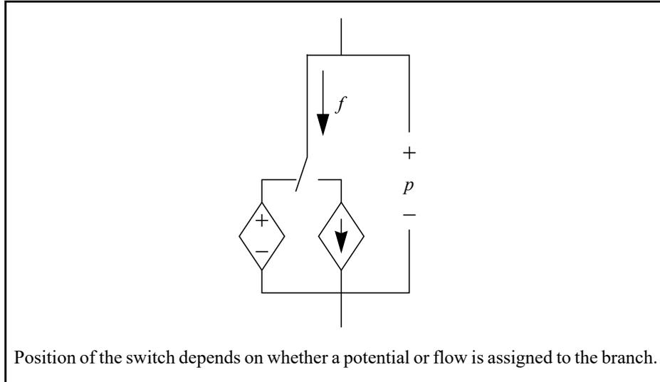
**Figure 5-5: Circuit model for a switched source branch**
