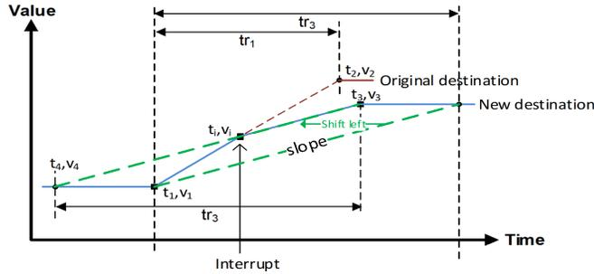
**Figure 4-8: Interrupted rising transition (rising  $tr_3 > tr_1$ )**
