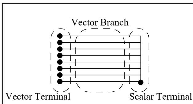
**Figure 3-2: One vector and one scalar terminal**
