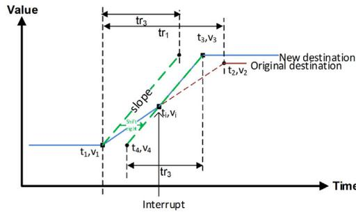
**Figure 4-9: Interrupted rising transition (rising  $tr_3 < tr_1$ )**
