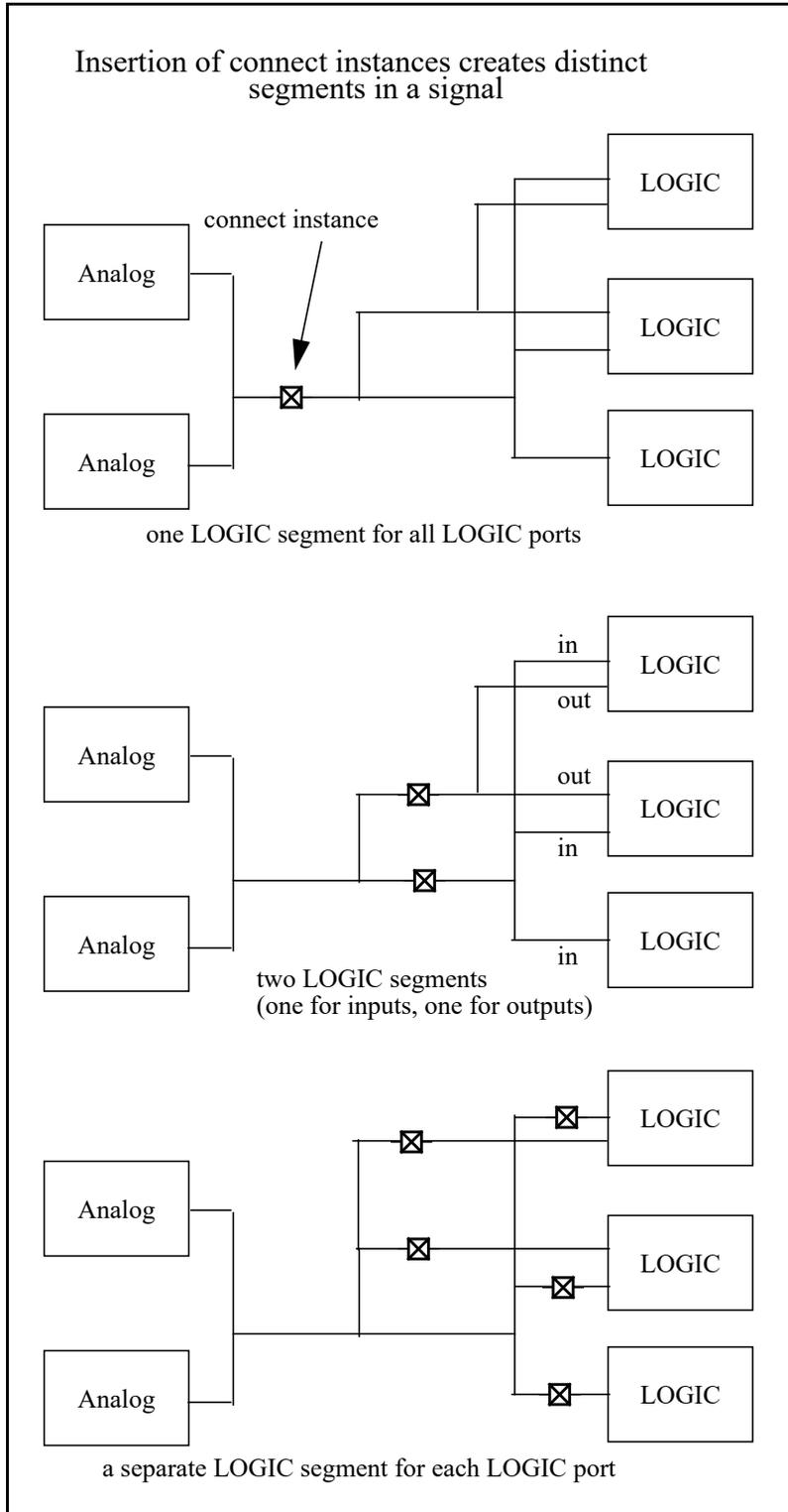
**Figure 7-7: Signal segmentation by connect modules**
