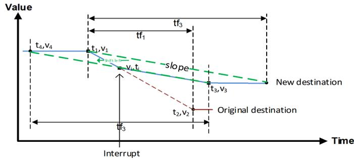
Figure 4-10: Interrupted falling transition (falling  $tf_3 > tf_1$ )
