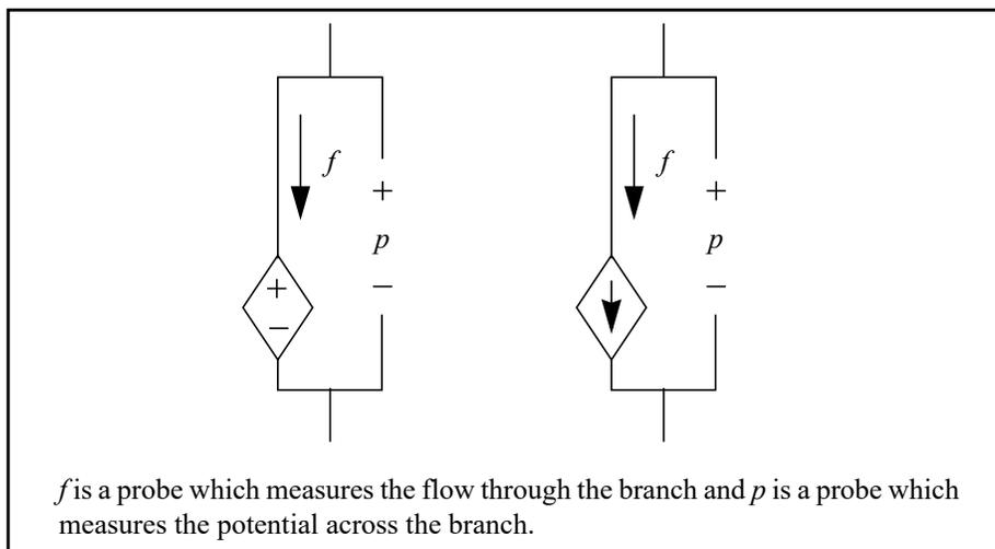
**Figure 5-2: Equivalent circuit models for source branches**
