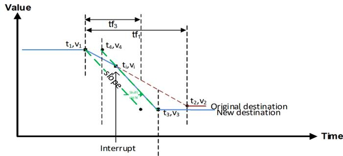
Figure 4-11: Interrupted falling transition (falling  $tf_3 < tf_1$ )
