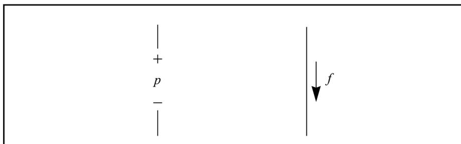
Figure 5-1: Equivalent circuit models for probe branches
