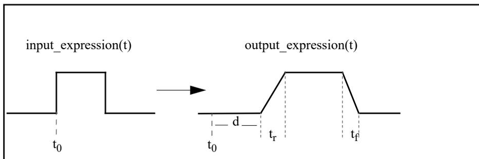
Figure 4-5: Transition filter example
