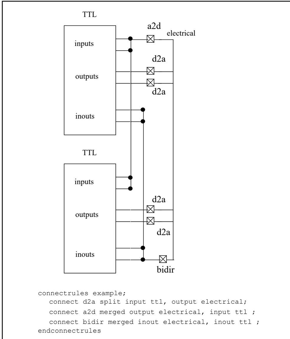
**Figure 7-10: Connect module insertion with signal segmentation**
