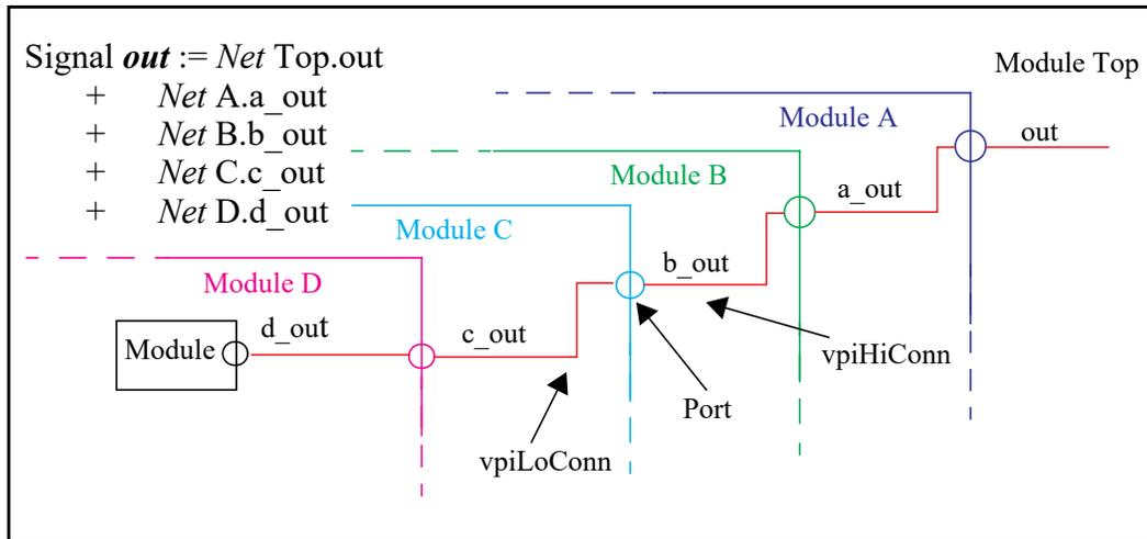
Figure 7-1: Signal “out” hierarchy of net segments
