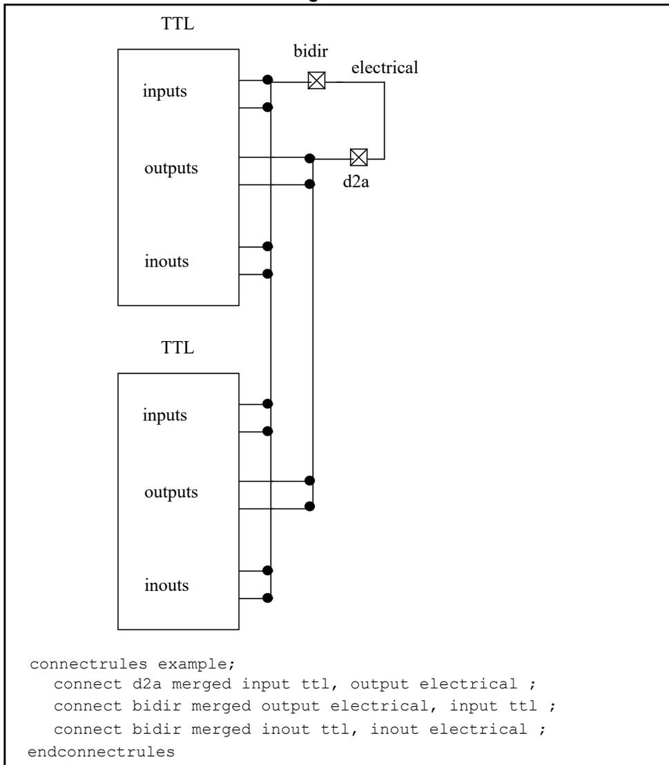
Figure 7-9: Connector insertion using merged
